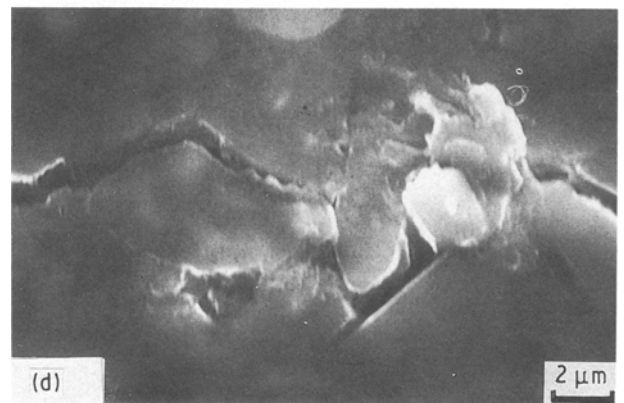
Figure 5 Characteristics of cyclic fatigue cracks in AD 90 alumina. (a) Typical profile of the fatigue crack. (b) Roughness-induced crack closure. (c, d) Debris particles and glass phase being squeezed out of the crack by the pumping action of the crack walls under cyclic loading.
